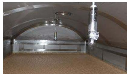
**After:** A cleaned fermentation tank with Alfa Laval GJ PF FT tank cleaning machines.
