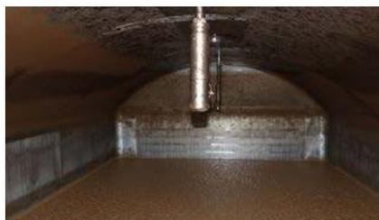
**Before:** Dirty fermentation tank with Alfa Laval GJ PF FT tank cleaning machines.
